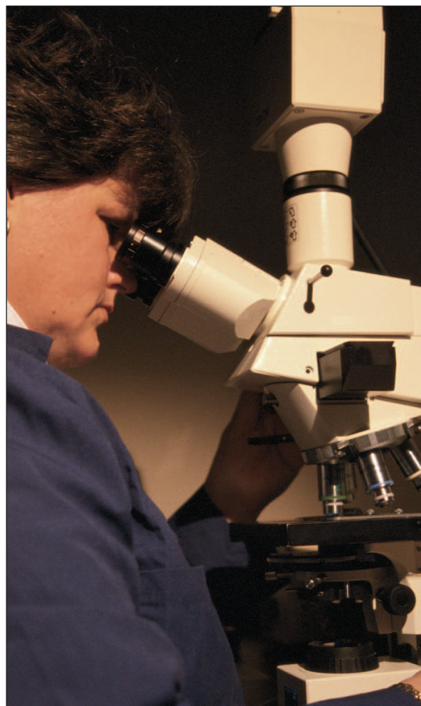
Microscopist quantifies excystation of Cryptosporidium oocysts before exposure to UV light.
