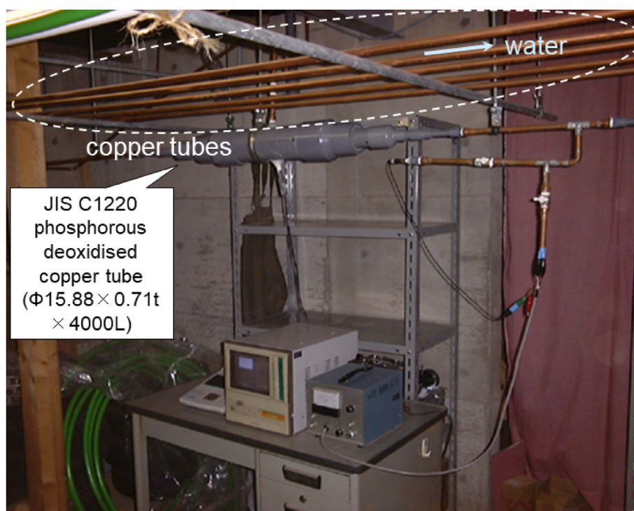
Figure 2. Appearance of field test system installed in the basement of a local plumbing contractor. Five copper tubes measuring 4000 mm in length were connected with brazing joints, and the water inside the tubes was replaced once per week.
