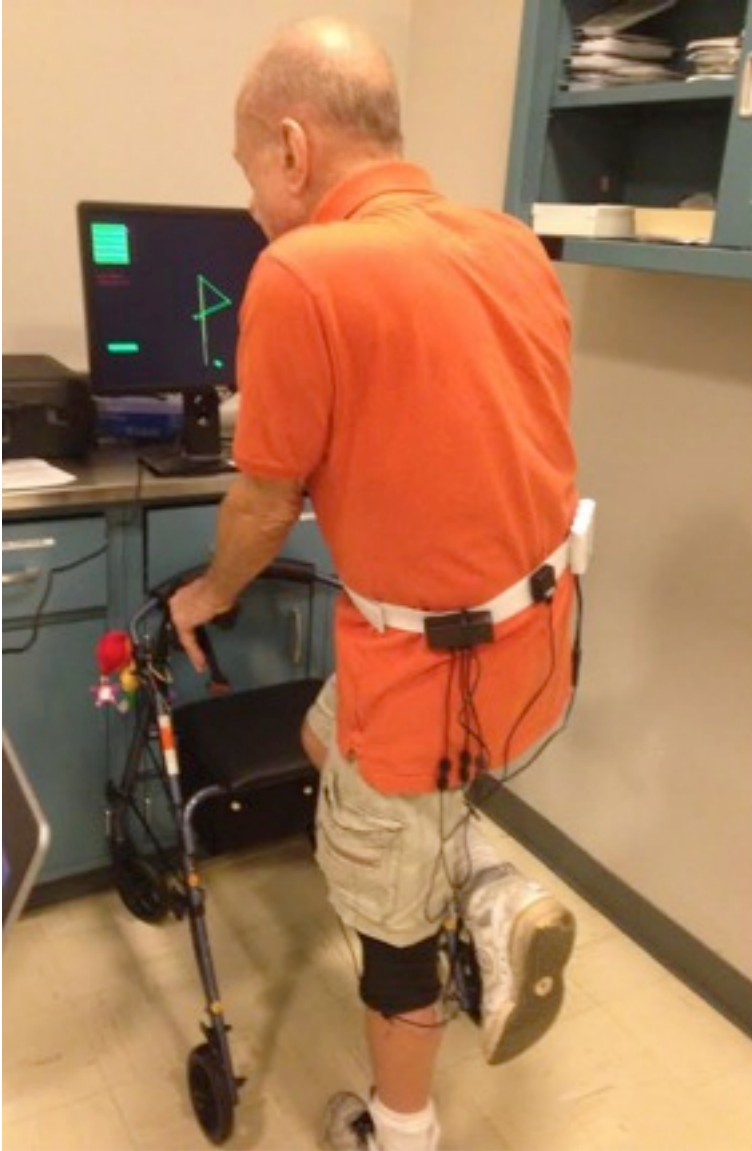
Figure 2: Subject Performing Obstacle-crossing Task with Support of Walker. The subject sees only his lower limbs on the screen and alternates moving his legs to avoid hitting the virtual obstacle displayed on the screen. The individual gave written consent to being photographed.
