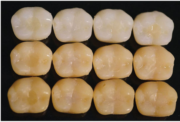
Figure 2. Representative images of different colored plastic crowns with composite restorations for visual color matching analysis. From left to right: G1A, G7A, Omnichroma, Filtek Supreme (shade A3). Shades from up to down: A1, A3, A4.
