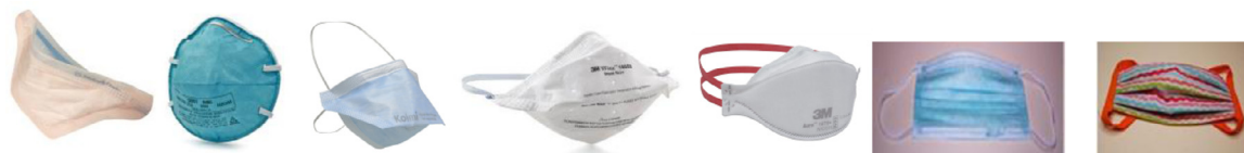
Fig 1. Panel of N95 respirators, Medical Masks (MM) and a community cloth mask tested. From left to right: Halyard Fluidshield Duckbill 46,727 N95 respirator, 3M 1,860 N95 respirator, Kolmi Duckbill Filtering Face Piece (FFP) 2 NR Type 2R, 3M VFlex 1804 N95 respirator, 3M 1,870 + N95 respirator, EN 14,683 Type 2 medical mask (generic), cloth community mask.
