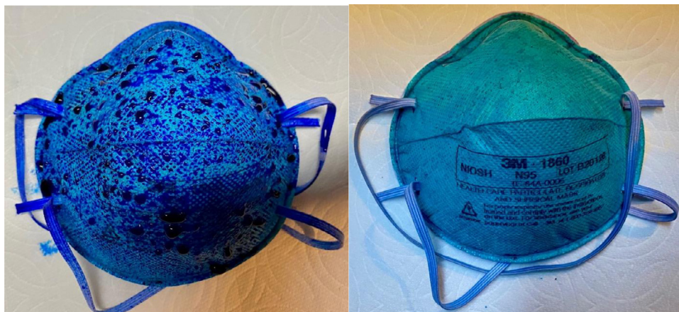
Fig 3. Sprayed and dried N95 respirator. Example of mask immediately after MB spray application with 1,000 \mu M MB (left) and after drying for 24 hours (right). MB is visible to the unaided eye on the respirator but with less intensity compared to immediately after application.
