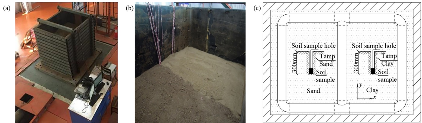
Fig 3. Preparation of test soil and preparation of soil sampling for soil parameters. (a) Laminar shear box, (b) The division of sand and clay, (c) Schematic diagram of soil sampling.
