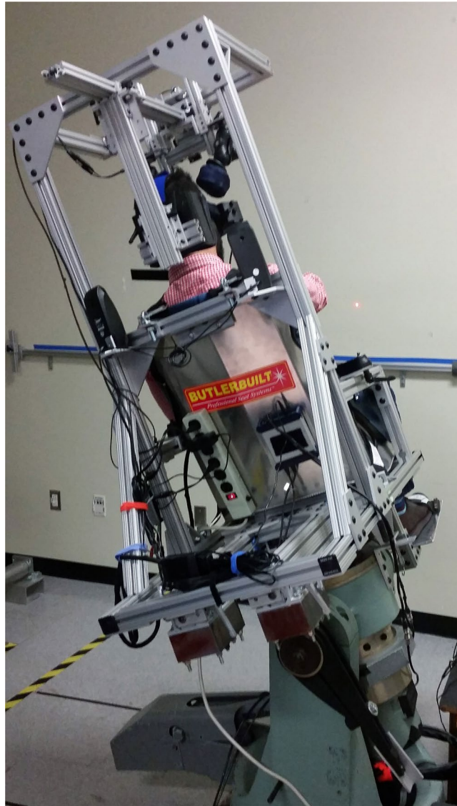
Figure 2. The NASA Johnson Space Center Off-Vertical Axis Rotation chair was used to tilt the ISS crewmembers 25° to the right or to the left.
