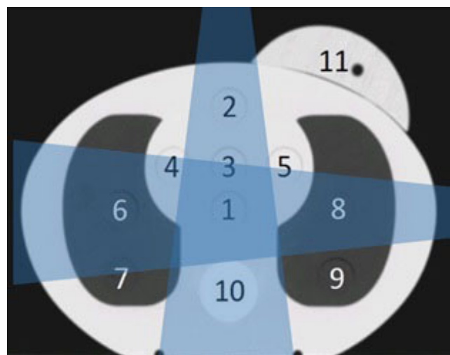
FIG. 1. Anthropomorphic phantom (CIRS) with dose measurement points and isocenter locations identified. Point 11 is offset by 5.5 cm longitudinally from points 1–10. In this study, isocenter was located at point 1, 2, 6, 8, 10 and 12, which is in the center of the phantom with an 8 cm offset from the axial plane of points 1–10. The target region of MV-MV is illustrated as dark blue (intersection) region. The remaining part is defined as extra-target region.
