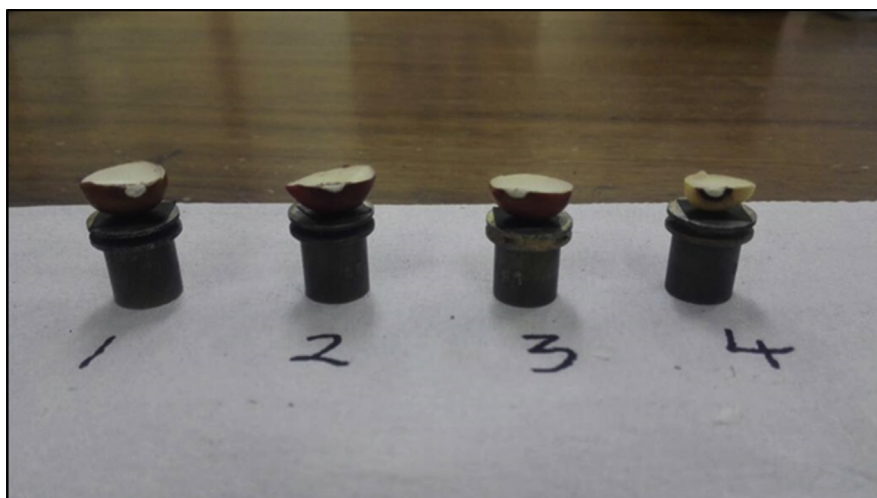
Fig. 1. Fixed and embedded seed of Bambara groundnut landraces mounted on stubs (1) Mana, (2) G340A, (3) Kazuma, and (4) Kazai. EDX analysis for the three seed regions of each Bambara landrace was done using a Zeiss EVO Ls15 scanning electron microscope (SEM) connected to a spectrometer (EDAX model 808A) detector, and an INCA microanalysis suit (ETAS Group). All analysis work took place at a speeding up voltage of 5 kV and working distance (WD) of 7.5 mm. Each analysis lasted 60 seconds in duration. To lessen equipment-caused variation, the EDX electronics were turned on 15 minutes before use, the filament of the SEM was kept aligned and the count rate was adjusted to 1200 counts/sec. Using the INCA window system, integrated counts under the Ca, K, Mg, P, Mn, Zn, Fe, and Cu peaks were determined. After peak values were determined the spectra were then automatically put through by INCA program.
