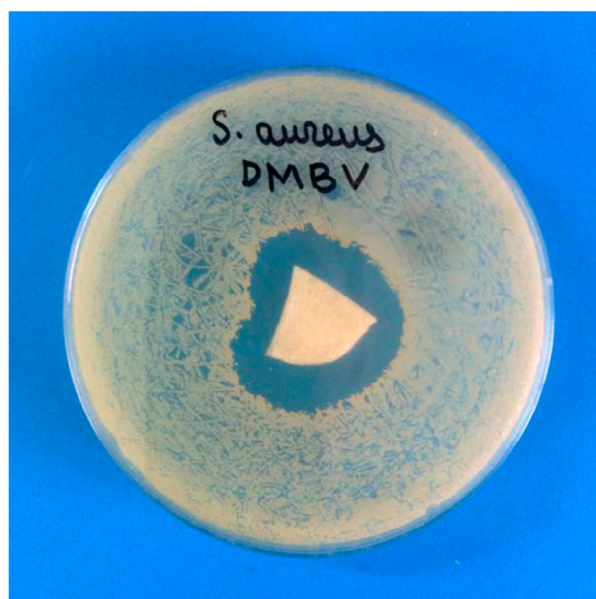
Figure 7. The result of the diffusion test, which demonstrates the formation of the zone of inhibition of the growth of bacteria Staphylococcus aureus caused by the release of vancomycin from the Ca-alginate sponge.
