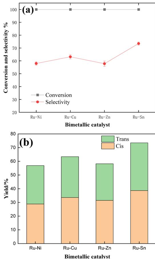
Fig. 9 (a) Conversion and selectivity of different bimetallic catalysts, and (b) the *cis-trans* ratio of the products. <sup>a</sup>Reaction conditions: reaction temperature 120 °C, reaction pressure 4 MPa, reaction time 1 h, 40 mL of tetrahydrofuran solution containing 3% TMCB, and catalyst 0.5 g.
