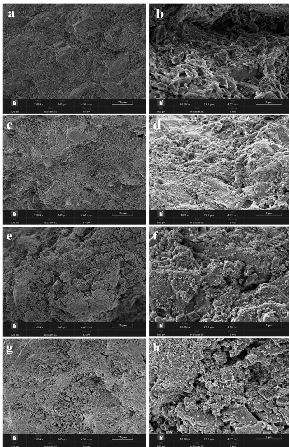
Fig. 4 Scanning electron microscopy map of the Ru-Sn/Al<sub>2</sub>O<sub>3</sub> catalyst: (a and b) Ru : Sn = 2 : 1; (c and d) Ru : Sn = 1 : 1; (e and f) Ru : Sn = 1 : 2; (g and h) Ru : Sn = 1 : 3.
