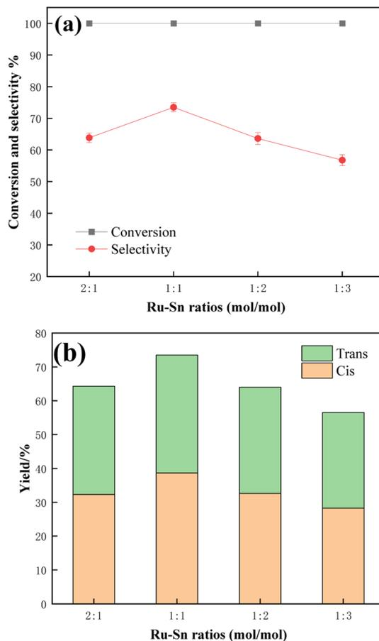
Fig. 10 (a) Conversion and selectivity of catalysts with different Ru-Sn ratios, and (b) the *cis-trans* ratio of the products. <sup>a</sup>Reaction conditions: reaction temperature 120 °C, reaction pressure 4 MPa, reaction time 1 h, 40 mL of tetrahydrofuran solution containing 3% TMCB, and catalyst 0.5 g.
