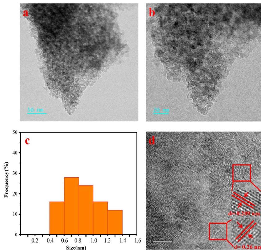
Fig. 7 (a and b) 1 : 1 the TEM of the Ru-Sn/Al<sub>2</sub>O<sub>3</sub> catalyst (c) particle size distribution and (d) HRTEM.
