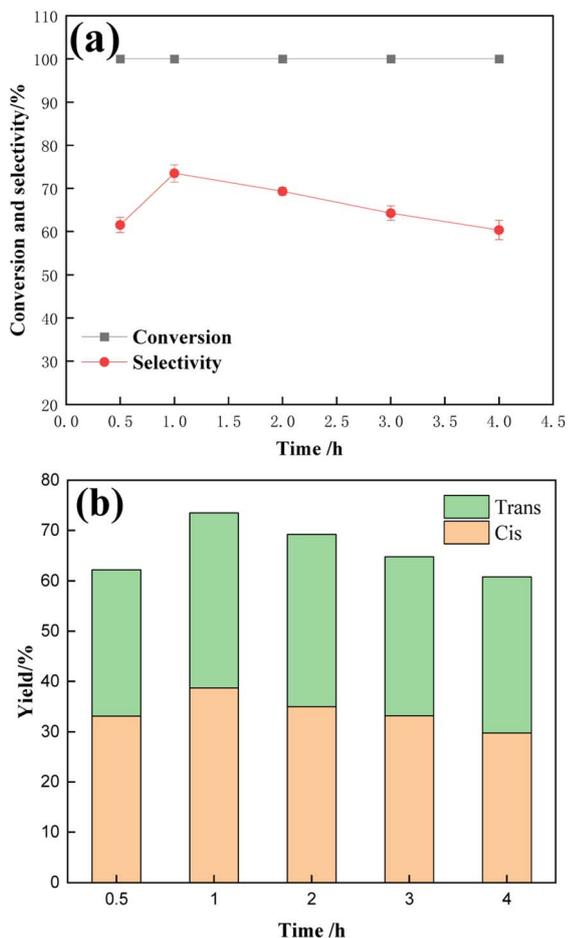
Fig. 13 (a) Conversion and selectivity at different times, and (b) the *cis-trans* ratio of the products. <sup>a</sup>Reaction conditions: reaction temperature 120 °C, reaction pressure 4 MPa, 40 mL of tetrahydrofuran solution containing 3% TMCB, and catalyst 0.5 g.
