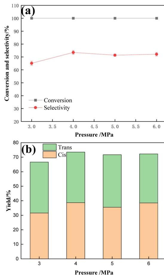
Fig. 12 (a) Conversion and selectivity at different pressures, and (b) the *cis-trans* ratio of the products. <sup>a</sup>Reaction conditions: reaction temperature 120 °C, reaction time 1 h, 40 mL of tetrahydrofuran solution containing 3% TMCB, and catalyst 0.5 g.
