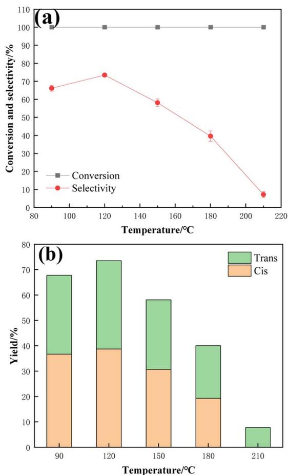
Fig. 11 (a) Conversion and selectivity at different temperatures, and (b) the *cis-trans* ratio of the products. <sup>a</sup>Reaction conditions: reaction pressure 4 MPa, reaction time 1 h, 40 mL of tetrahydrofuran solution containing 3% TMCB, and catalyst 0.5 g.
