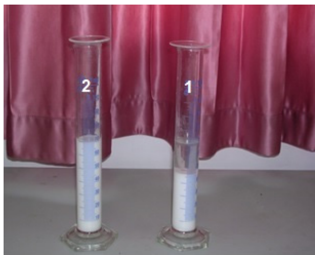
Figure 13. Phase separated original drug “Maalox” (1) and phase stable “Maalox” containing 2% of ANC (2).
