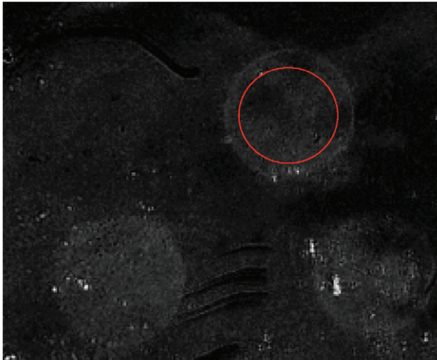
Figure 2. Difference images obtained from SPRi of antibodies binding to GAD65 immobilised at a gold/GLISS surface. Spots (400 \mu\text{m} diameter) containing GAD65 protein were immobilised by spotting at the surface using Hamilton Starlet equipped with a PinTool tip and modified software. GAD1 antibody (4.8 nM in 200 \mu\text{l} PBS) was flowed across the surface at 20 \mu\text{l}/\text{min} as described in Methods and differential images obtained using the GenOptics SPRi device. The red circle illustrates the area that is generally chosen to calculate the pixel density at any given time in order to generate curves of the type shown in Figure 3.
