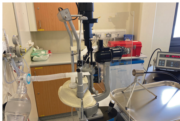
Fig. 1 Photograph of the experimental setup. The nebuliser particle source and optical particle detector can be seen either side of the slit lamp.
