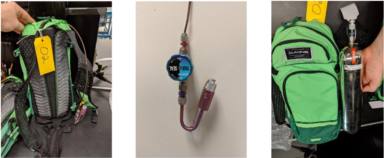
Figure 1. Consumer sampling backpack containing an evacuated steel canister, sampling line, flow regulator and start/stop knob, and MSR climate monitor.
