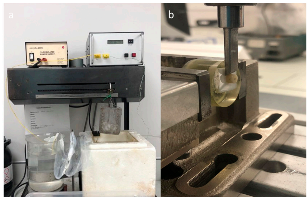
Figure 5. Bonded specimens underwent 10,000 thermocycles between 5 °C and 55 °C (a) before being tested for shear bond strength (SBS) (b).
