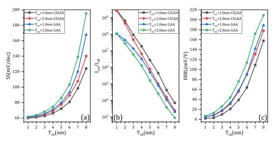
**Figure 7.** The simulation results of CIGAA and GAA: (**a**) subthreshold slope (SS) of CIGAA and GAA; (**b**) switching ratio  $(I_{on}/I_{off})$  of CIGAA and GAA; (**c**) drain-induced barrier lowering (DIBL) of CIGAA and GAA. All three of the figures are plotted when  $D_{CI} = 4.0$  nm.
