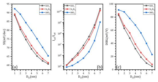
**Figure 9.** The simulation results of CIGAA and GAA in terms of different Core–Insulator material and  $D_{CI}$ : (a) subthreshold swing (SS); (b) switching ratio  $(I_{on}/I_{off})$ ; (c) drain-induced barrier lowering (DIBL). All three figures are plotted when  $D_{NW}$  is fixed to 8 nm.
