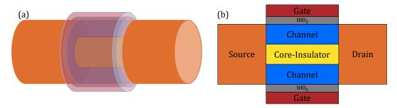
**Figure 1.** The schematic 3D structure and cross section of CIGAA: (a) 3D view of CIGAA; (b) cross-sectional view of CIGAA. The illustrations are not depicted proportionally to the really devices; we made some exaggeration for a clear visualization.
