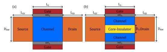
**Figure 2.** The overall dimension of CIGAA and GAA: (**a**) parameters used for GAA; (**b**) parameters used for CIGAA.
