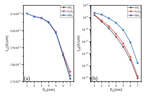
**Figure 8.** The simulation results of CIGAA and GAA in terms of different Core–Insulator material and  $D_{CI}$ : (a) on-state current. (b) off-state current. Both figures are plotted when  $D_{NW}$  is fixed to 8 nm.
