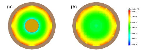
**Figure 5.** The electron density plot of CIGAA and GAA, the devices are at on state: (**a**) electron density of GAA; (**b**) electron density of CIGAA. Both figures are plotted when  $V_{GS} = V_{DS}$ ,  $V_{DS} = 1$  V. Metal gate and part structures are not included in the figure for clarity.
