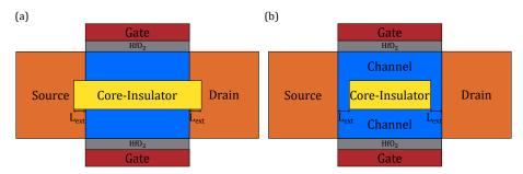
**Figure 10.** The illustrations which show the issue of Core–Insulator's extension and contraction: (**a**) the Core–Insulator extends itself into source and drain by  $L_{ext}$ ; (**b**) the Core–Insulator recesses itself into channel by  $L_{ext}$ .
