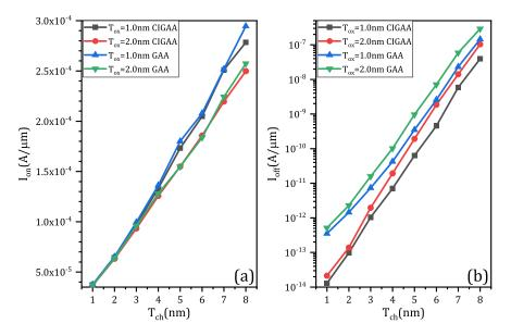
**Figure 4.** The simulation results of CIGAA and GAA: (**a**) on-state current ( $I_{on}$ ) of CIGAA and GAA; (**b**) off-state current ( $I_{off}$ ) of CIGAA and GAA. Both of the two figures are plotted when  $D_{CI}$  = 4.0 nm.
