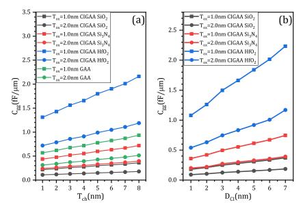
Figure 11. Gate capacitance dependence on: (a) channel thickness; (b) the Core–Insulator diameter D<sub>CI</sub>.
