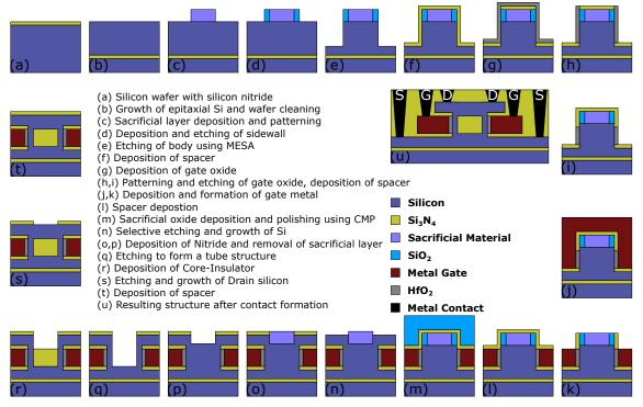
Figure 3. Suggested fabrication process flow for CIGAA.
