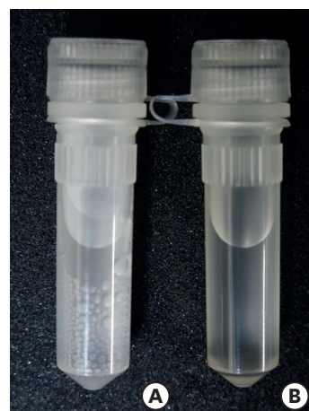
Figure 2. The formation of chlorine gas bubbles in the mixed solutions. (A) 17% EDTA and 5% NaOCl, (B) 1% IP6 and 5% NaOCl.
