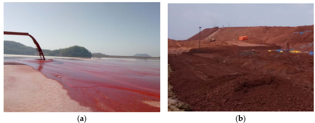
Figure 1. Discharge and stacking of red mud. (a) Mud treatment. (b) Dry mud treatment.
