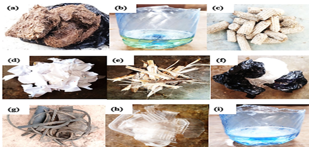
Figure 3. Ignition aids (a) Oguso, (b) petrol, (c) maize cob, (d) paper (printed-on type), (e) wood, (f) nylon, (g) rubber, (h) plastic, (i) kerosene ( source: present study, 2022).
