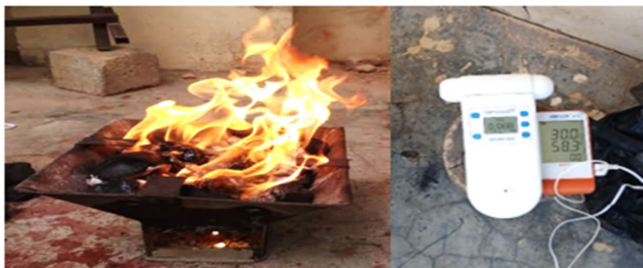
Figure 4. Measurement of combustion indices from a typically loaded charcoal pot ( source: present study, 2022).
