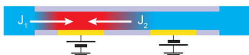
Figure 7. Fluxes of reduced molecules to the generator electrode: J_1 from the bulk solution outside the nanogap device and J_2 from the collector electrode via redox cycling.
