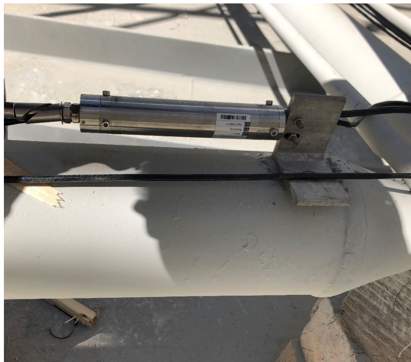
Figure 4. Horizontal single-axis inclinometer.
