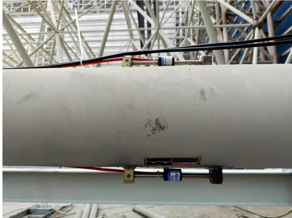
Figure 7. A vibrating wire surface strain gauge.
