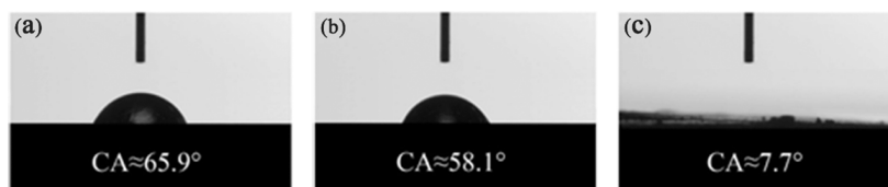
Figure 6. Contact angle on the surface of (a) HPMoV-VIM, (b) HPMo-VIM, and (c) HPW-VIM.
