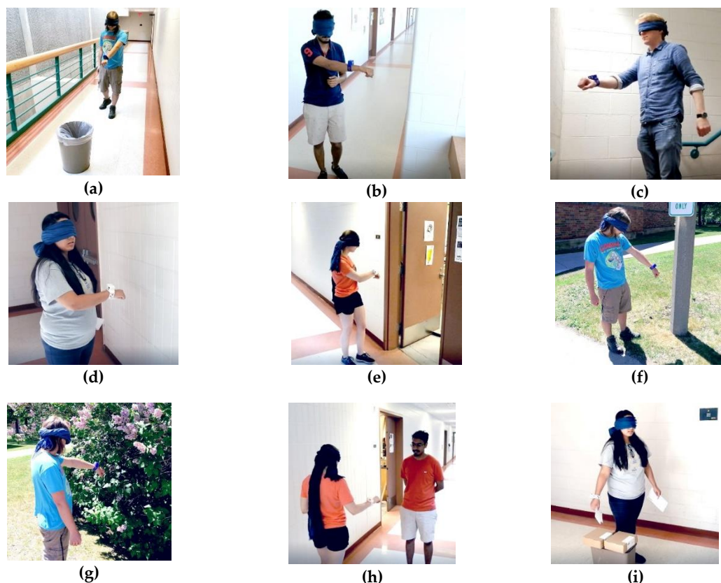
Figure 6. Testing procedure. (a) Walk along the corridor with an unknown obstacle; (b) Bypass several corners indoors; (c) Walk through the staircase; (d) Wall following; (e) Detect the open door; (f) Detect an obstacle on the street; (g) Bypass an obstacle on the street; (h) Avoid collisions with pedestrians; (i) Interact with known objects.
