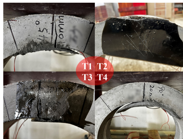
Figure 9. Liner–pipe interfaces after TEBTs of T1–T4.
