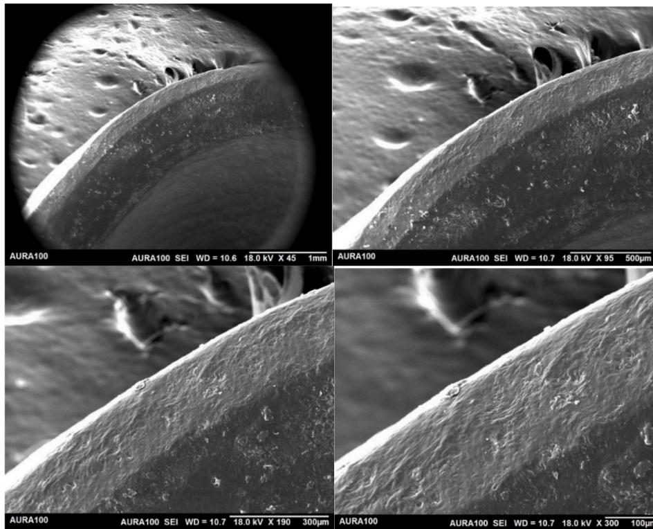
Fig. 5. SEM images of crown margins milled at different magnifications. From left to right: 45×, 95×, 190×, and 300 × magnification.
