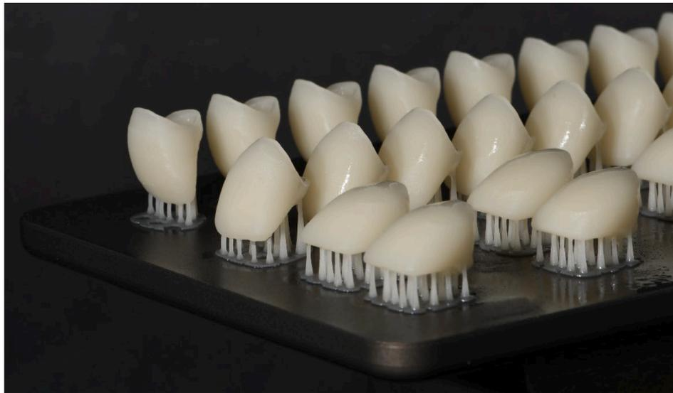
Fig. 1. Additive manufacturing samples positioned at their relative orientations on the printing platform immediately after printing using temporary crown and bridge material (Freeprint temp, Detax Ettlingen, Germany).
