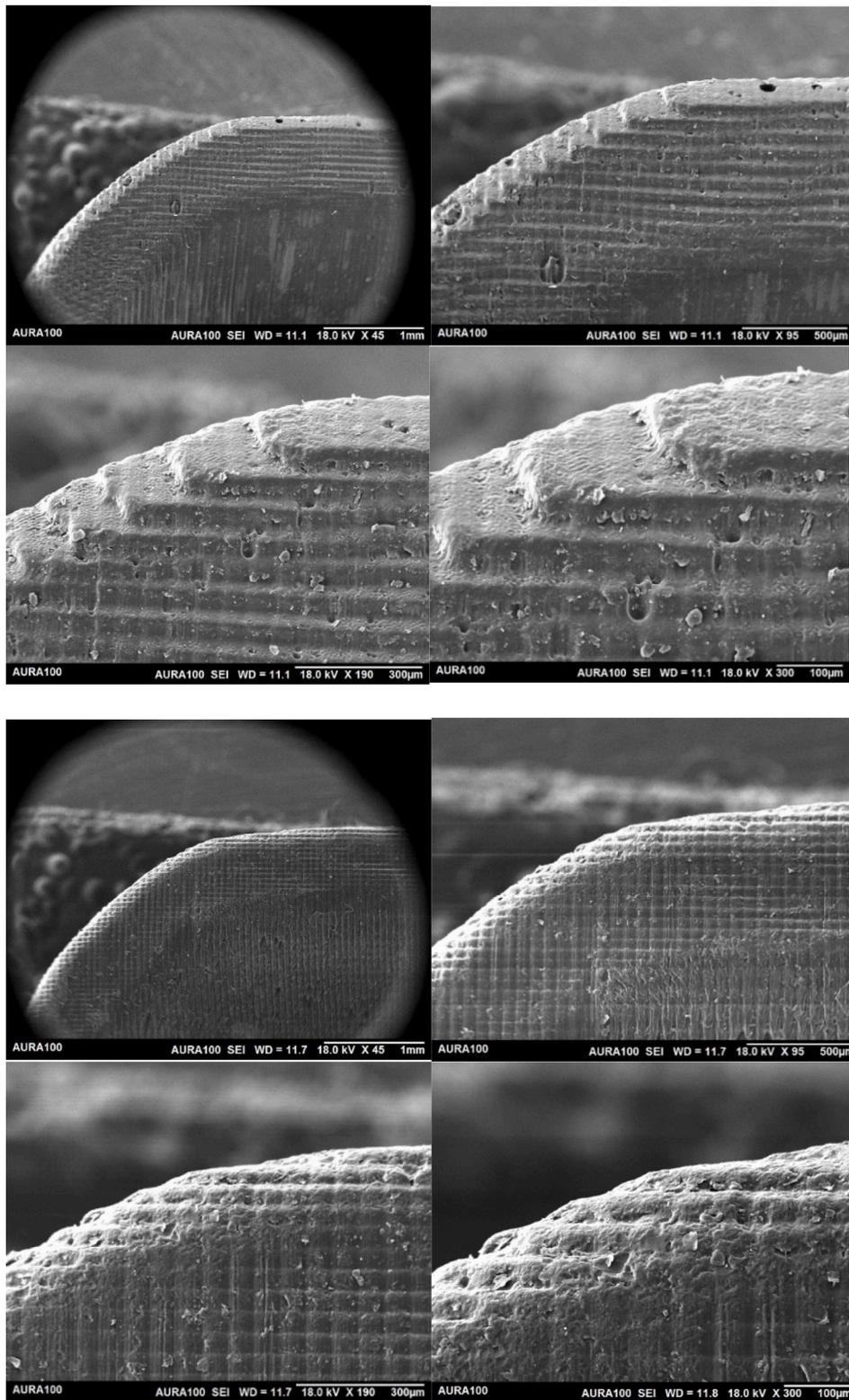
Fig. 4. SEM images of crown margins 3D printed at 90° (Top 4 images), 45° (middle 4 images), and 0° (bottom 4 images) at different magnifications. From left to right: 45×, 95×, 190×, and 300 × magnification.
