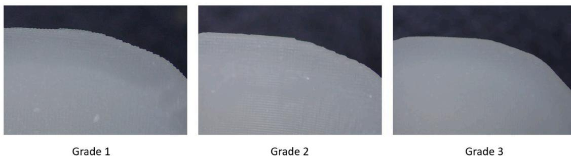
**Fig. 2.** Margin quality grading system. Grade 1: rough boundaries appearing as steps or layers. Grade 2: slightly rough boundaries with fewer irregularities. Grade 3: smooth and continuous boundaries.
