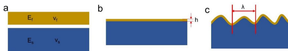
Figure 3. Schematic diagram of the plane wrinkling. (a) A planar double-layer hard and soft system, (b) the system in stretching mode and (c) the system in released mode.
