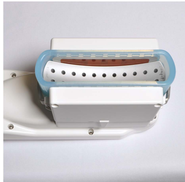
Figure 1. Prototype CoolCup was created by inserting a machined metal cup into a modified parallel plate cryolipolysis applicator.
