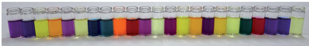
Fig. 5 Photographic demonstration of fine color-tuning with aminoanthraquinone-based dyes with 1 – 23 (arranged by compound number from the left).
