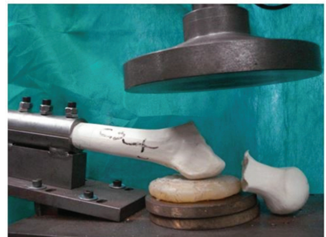
Fig. 4 Experimental model after fracture.
