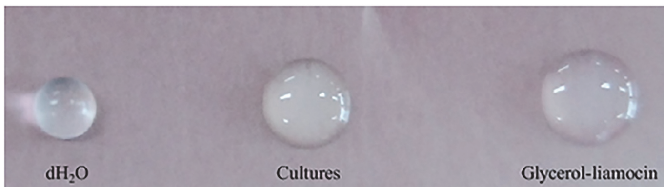
Fig 5. Picture illustrating the surface tension of glycerol-liamocin in aqueous solution dropped on a hydrophobic film.
