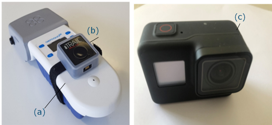
Fig. 2. The utilised sensors used: PM10 and PM2.5 (a), GPS iTrail (b) and GoPro (c).
