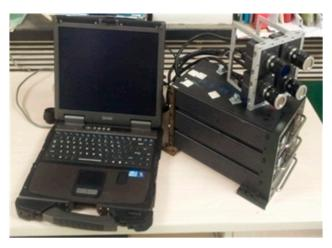
Figure 1. The four-camera multispectral mapping system.
