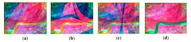
Figure 19. The CIR composite of the four-band images;  $(\mathbf{a}-\mathbf{c})$  respectively the multispectral images obtained by using the methods using the first-order polynomial, second-order polynomial and homography model and using the RANSAC directly; (d) the multispectral images obtained by using our method.
