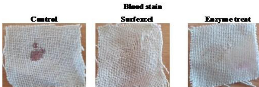
Fig. 3. Application of protease produced by Bacillus halodurans on the removal of blood stain.
