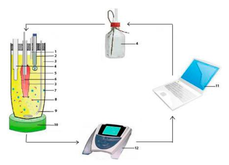
**Figure 1.** The new lipolysis-absorption model for lipid-based formulations: (1) Vent; (2) pH electrode; (3) intestinal tissue medium; (4) NaOH autoburette; (5) intestinal segment; (6) sampler; (7) a lipid-based formulation; (8) pancreatic lipase/colipase; (9)  $O_2/CO_2$ ; (10) temperature controlled stirrer; (11) computer; and (12) pH-stat meter controller.
