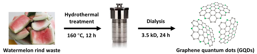
Figure 1. Preparation of GQDs from watermelon rind waste through the hydrothermal technique.
