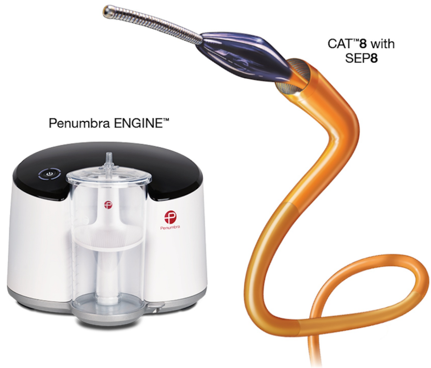
FIGURE 4: Picture of the Penumbra Indigo® Aspiration System showing the CAT™8, SEP™8, and ENGINE™. The CAT™8 (size: 8-French/2.67 mm diameter, 85 cm length) is the suction catheter used to remove the clot. The separator (SEP™8) allows the user to macerate the clot if necessary while aspirating it through the lumen of the CAT™8. The ENGINE™ powers the vacuum and collects the aspirated clots. Image reproduced with permission from Penumbra Inc. (Alameda, CA, USA).
