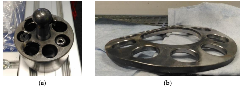
Figure 1. The damaged parts of an axial piston pump: (a) cylinder block with pistons, (b) slipper-retainer.
