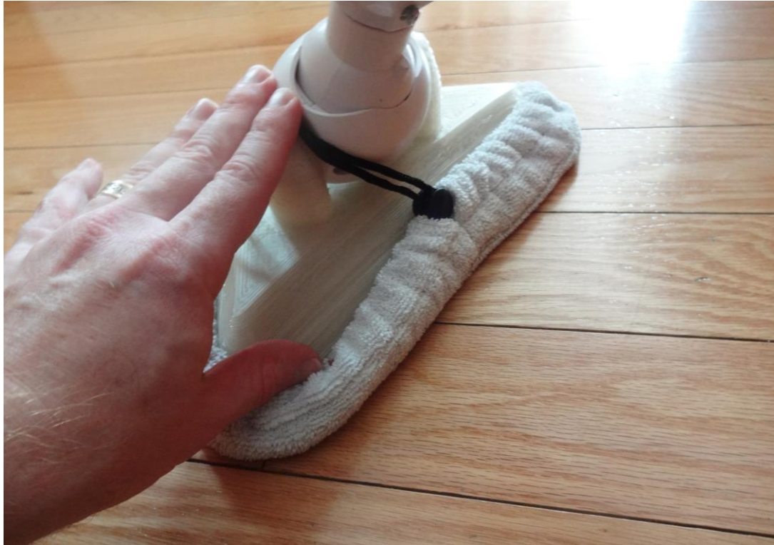
Figure 9. Waste PC 3D-printed steamer head shown assembled on steamer.
