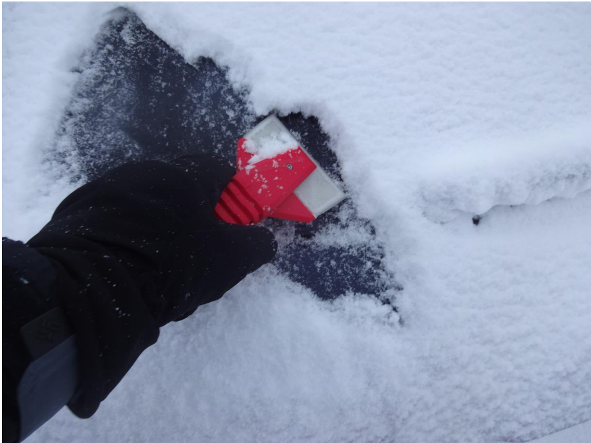
Figure 11. 3D-printed ice/snow scraper in use. The blade is recycled PC and the handle is polyactic acid (PLA).
