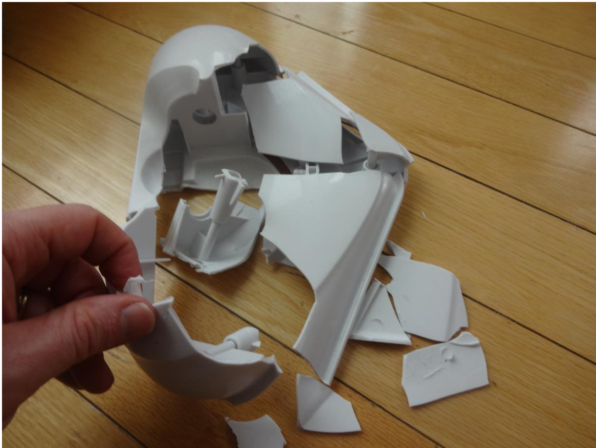
Figure 7. Broken commercial proprietary steamer head. The plastic became brittle and disintegrated under normal use.
