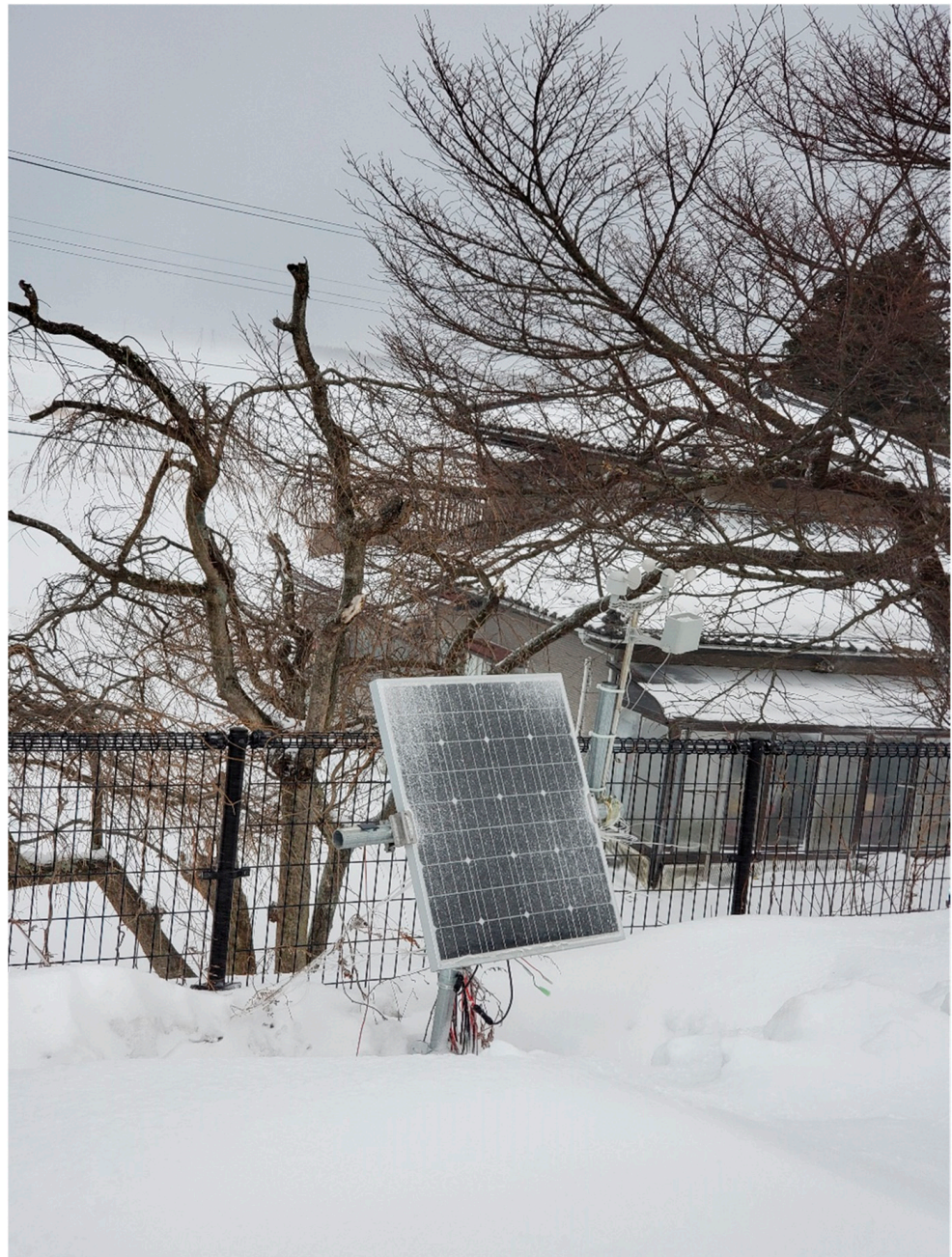
Figure 19. KOSEN-WS set up in Tsuruoka (outdoors) during winter. There is a significant amount of snow around the KOSEN-WS, but the KOSEN-WS is operating continuously.
