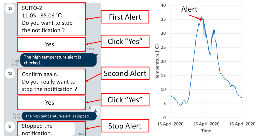
Figure 21. An example of alert notification at high temperature. The alert notification is sent to farmers’ smartphones using LINE when the temperature is over 35 °C. The figure on the right shows an alert notification by LINE. The user needs to click “Yes” after the first alert notification is received. After the second alert notification, the user needs to click “Yes” again. The user must click “Yes” twice to stop the alert notification. If the user does not confirm twice, the alert notification will continue to arrive.
