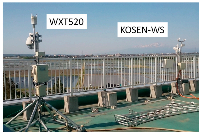
Figure 9. Installation locations of the KOSEN-WS and WXT520. The heights of the two airflow meters are the same, and the distance between the two devices is approximately 4 m.
