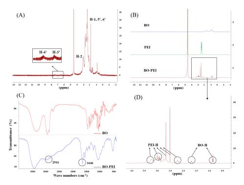
**Figure 1. (A)** Characterization of polyethyleneimine–folic acid (FA-PEI) copolymer by <sup>1</sup>H-NMR; **(B,D)** characterization of polyethyleneimine–borneol (BO-PEI) copolymer through <sup>1</sup>H-NMR spectroscopy; **(C)** characterization of BO-PEI copolymer through FTIR.
