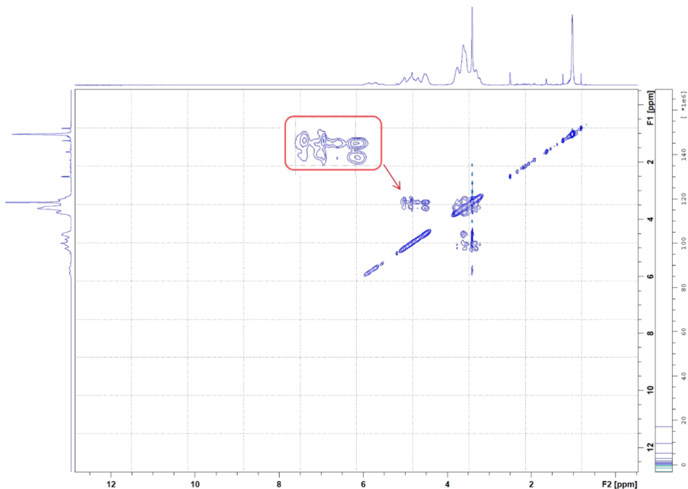
Figure 5. 2D-NOESY spectrum of PO-ICs in DMSO, demonstrating the interactions occurring between the PO protons and HP \beta CD protons inside the PO-ICs.
