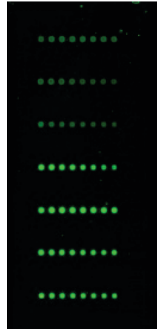
Figure 6 Calibration curve employed for determination of amounts of protein captured on the microarray surfaces. Specific amounts of purified GFP protein were printed on CodeLink activated slides. After incubation, fluorescent intensities were determined for each standard to create the calibration curve.
