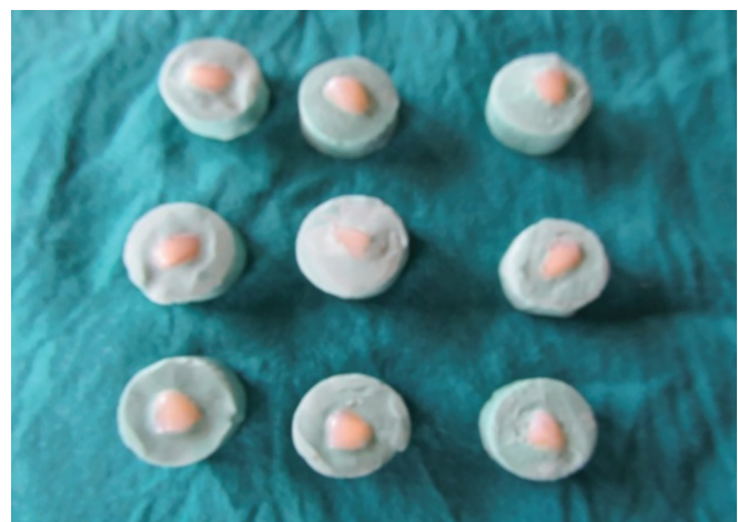
Fig. 4: Sectioned teeth mounted in dental stone
