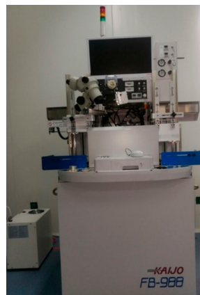
Figure 2. KAIJO FB-988 automatic wire bonder machine.
