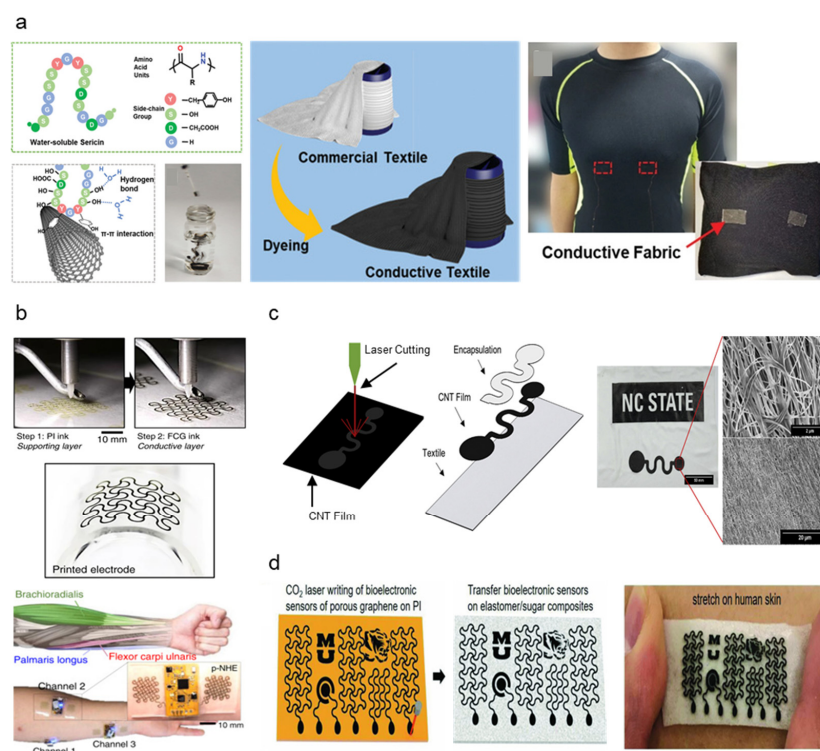
Figure 3. Carbon-based dry electrode fabrication and demonstration: (a) Chemical composition of SSCNT ink and fabrication procedure into conductive textiles (Reprinted with permission from Adv. Mater. 2020, 32, 2000165, Copyright 2020, Wiley) [55]. (b) Fabrication steps of PI and graphene ink onto stretchable nanomembrane surface and close-up image of the printed electrode (Reprinted with permission from Nat Commun. 2020 11, 3450, Copyright 2020, Nature Communications) [56]. (c) CNT electrode fabrication process via laser cutting and encapsulation, optical image of electrode microstructure transferred to the textile substrate (Reprinted with permission from Carbon 2020, 168, 673–683, Copyright 2020, Elsevier) [57]. (d) Porous LIG-based electrode fabrication on the soft substrate by laser writing and skin stretchability demonstration (Reprinted with permission from Adv. Mater. 2018, 30, 1804327, Copyright 2018, Wiley) [58].
