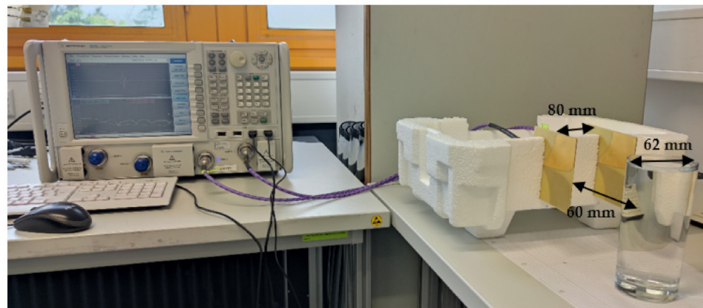
Figure 6. Proposed FD measurement setup.
