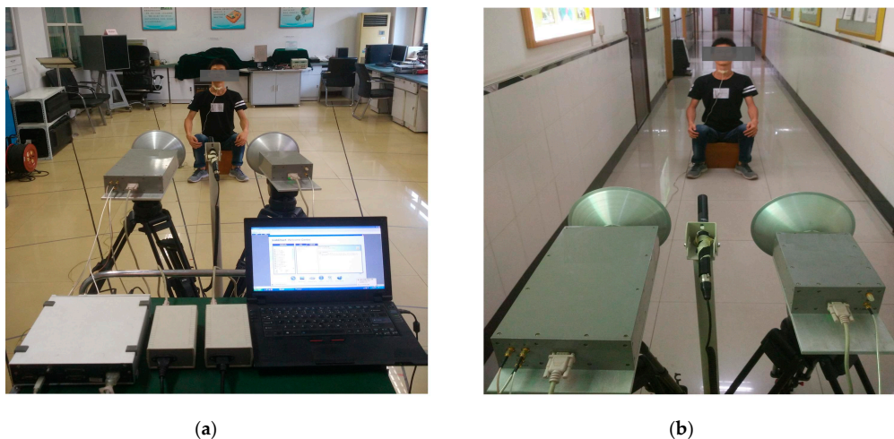
Figure 4. Experimental scenarios of the vocal vibration signal and acoustic signal detection: (a) enclosed room (2 m); (b) corridor (2 m).
