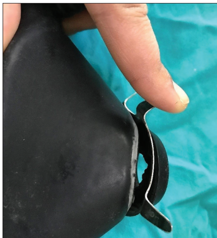
Figure 1: Mask showing tear at the junction of apex and body
