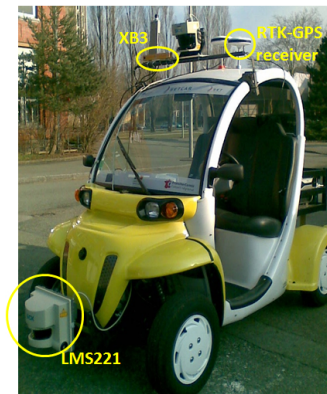
Figure 10. Equipped experimental platform.
